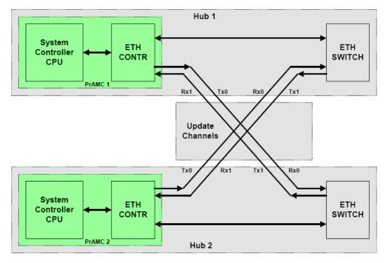
The block diagram shows one solution for the AMC GbE support channels with a PrAMC as System Controller.
